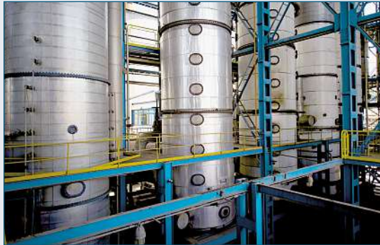
Ethanol made from sugar cane (above: harvesting; below: fermented sugar-cane juice flows through a series of distillation columns to produce ethanol)
