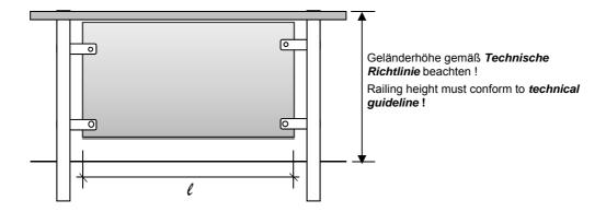
**Note:** If the types of glass and the dimensions listed in Table B are used, only static structural proof calculations are required.
